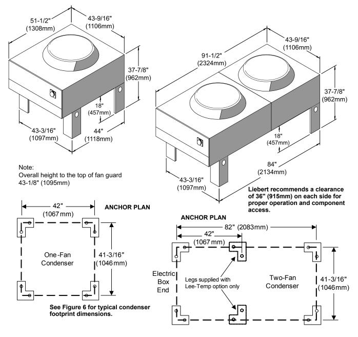
Figure 3 Condenser planning dimensional data—One-fan and two-fan units
